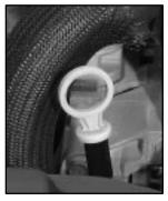
2.2L L4 ECOTEC (L61) Engine Check the oil here if you have a 2.2L L4 ECOTEC (L61) engine. The dipstick's handle will be a yellow ring. See "Engine Compartment Overview" in the Index for more information on location.
